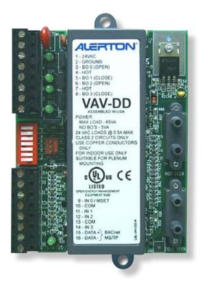
The Alerton® BACtalk® VAV-DD controller is a versatile, BACnet-compliant field controller that provides pressure-independent control of any dual-duct variable air volume (VAV) box. As a native BACnet controller, the VAV-DD integrates seamlessly with your BACnet system, communicating at up to 76.8 Kbps on a BACnet MS/TP LAN. The VAV-DD-F includes a filter to reduce dust contamination.
