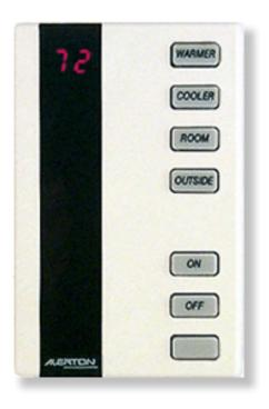
The Alerton® BACtalk® Microset™ is an intelligent zone temperature sensor with an optional humidity sensor. The Microset connects to Alerton's BACtalk VisualLogic® controllers (VLCs) and serves as a tenant control center and a field service tool as well as a sensor.
