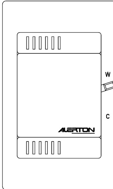
The Microtouch™ Wall Sensor is designed to complement any building's decor. The stylish housing contains a sensitive thermistor temperature sensing element, an override push-button switch, setpoint bias and a service jack for use with the Microset™ Service Tool.
